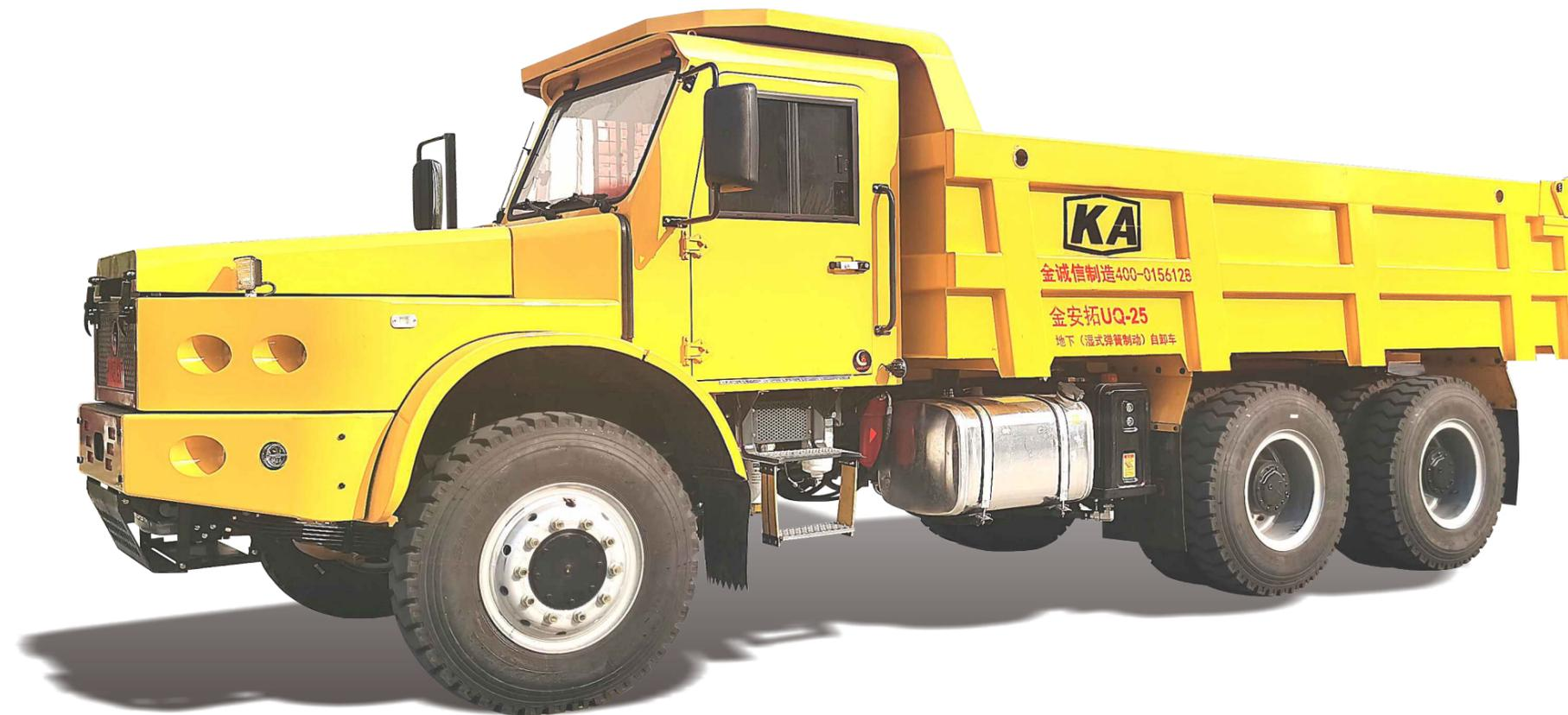
**UQ-25 (KAT25) Underground dump truck(Wet spring brake)**
