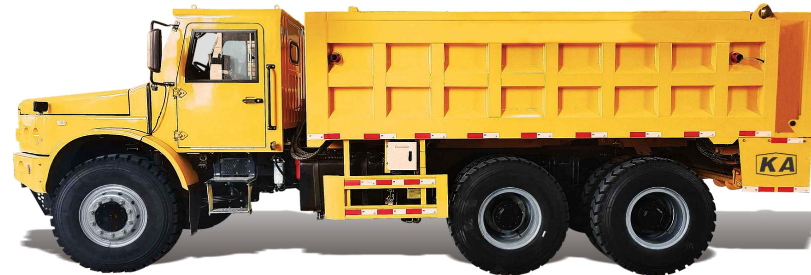
**KATUQ-25T underground dump truck (Wet spring brake)**
