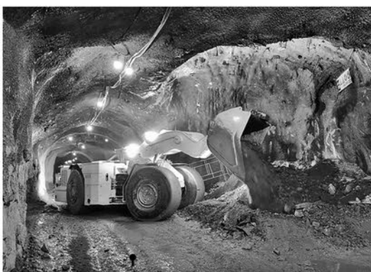
金川集团 (金川项目) | KAT614 地下内燃铲运机 DIESEL LOAD-HAUL-DUMP WORKING UNDERGROUND IN THE JINCHUAN PROJECT
