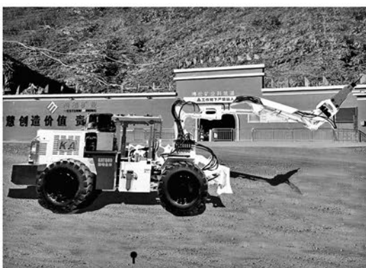
西部矿业 (肃北项目) | KATQ5 地下撬毛车 UNDERGROUND MECHANIZED SCALER WORKING UNDERGROUND IN THE SUBEI PROJECT
