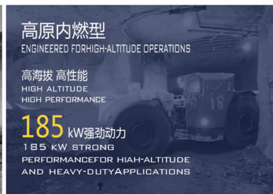
鑫源矿业 (白玉项目) | KAT307 地下内燃铲运机 (高原型) DIESEL LHD (HIGH-ALTITUDE MODEL) WORKING UNDERGROUND IN THE BAIYU PROJECT
