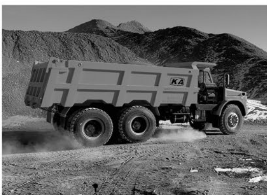
会宝岭铁矿 (会宝岭项目) | KATUQ-25 地下自卸车 UNDERGROUND DUMP TRUCK WORKING UNDERGROUND IN THE HUIBAOLING PROJECT
